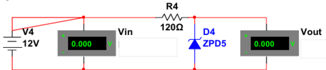
Gambar 3. Rangkaian reverse bias diode Zener
