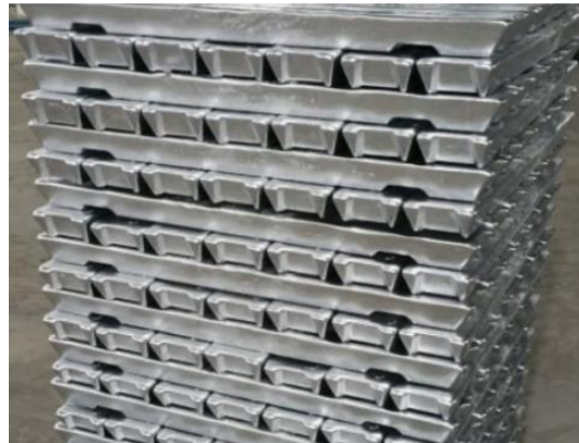
Gambar 5. Ingot Alumunium Ex Scrap Alumunium
