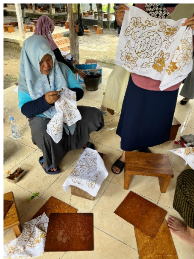
Figure 2 Original documentation from Giriloyo Batik Association craftsmen showing the nglowong process, which is the stage of coating the motif lines using canting.
